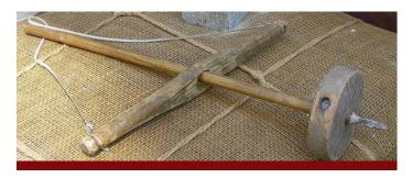
The same basic thing can be done with a pump drill. The only real difference between a pump drill and the bow drill is the way that the spindle is turned. Pump drills are harder, simply because the spindle has to be converted into a drill. To do this, a crossbar is needed, which has a hole that the spindle goes through. The string is attached to both ends of this crossbar, as well as run through a hole in the top of the spindle.
